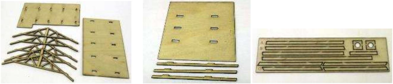
Glue the rafters to one half of the main roof, then add the other side. Because I wanted one half removable I taped it into position along the ridge, rather than glue it in place. The valances are applied next as in the photos. Make sure to leave a gap between the outermost rafters and the valance to allow for the wall.
