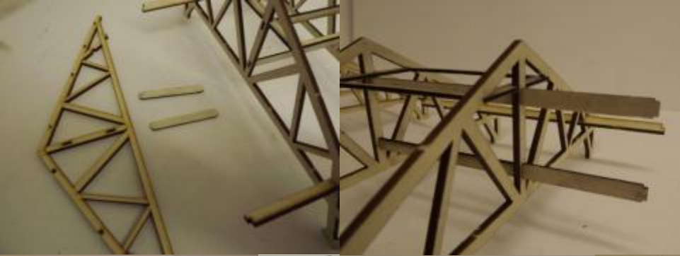
PHOTO 10D: join both halves of the roof frame together with centre A frame. Keep everything straight, square and level
