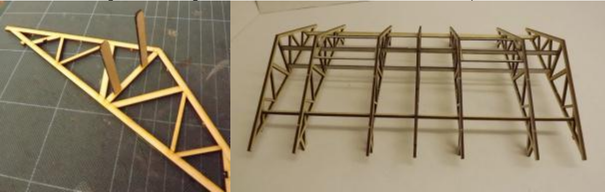
PHOTO 10F: Stain or paint the gable ends and glue to the frames.
