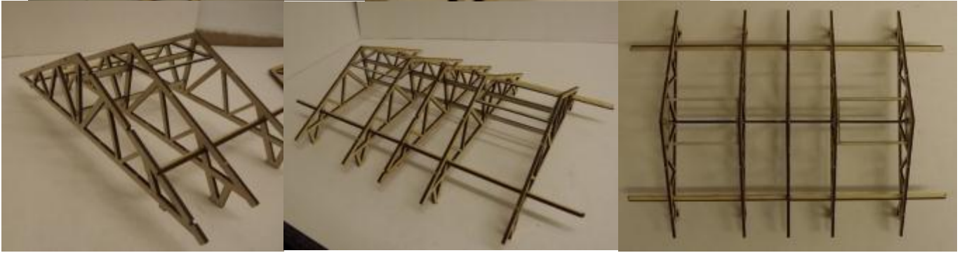
PHOTO 10E: using the remaining short centre bars, fit the end A frames to complete the frame structure.
