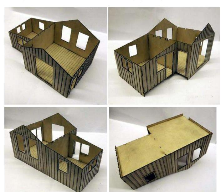
Now fit the corner trim to hide the slots. Again peel and stick parts, trimmed with some old cutters. (You can see the gap I left in the battens for the sliding door runners in the middle shot)
