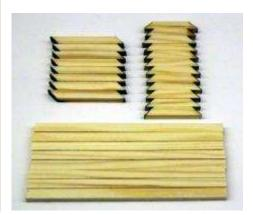
1.2 Remove the upper deck parts from their carrier and stain them. Glue the frame up as in the photos, ensure all is flat and angles are perpendicular. Its easiest to start with 6 inner pieces (use CA glue) then glue the rest.
